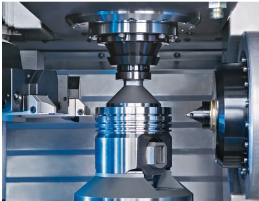
Machining a steel piston: plunge-cutting the grooves
