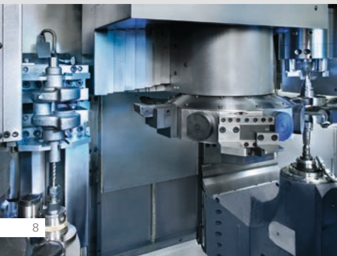
OP 10 + 20 Cutting to length, centring, turning (VTC 250 DUO)
