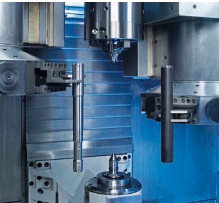
Component changeover: the finished component is removed and taken to its storage place; the new raw-part is loaded (sequence from right to left)
