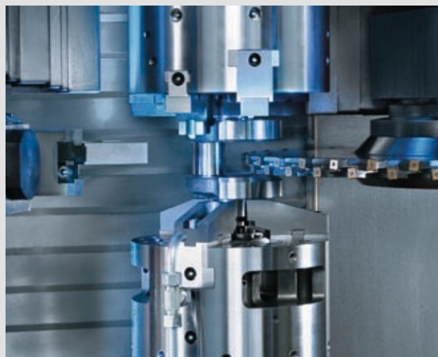
OP 30 milling the pin bearing (VTC 250 F)
