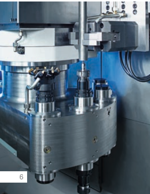
Shaft machining: centring and end machining
