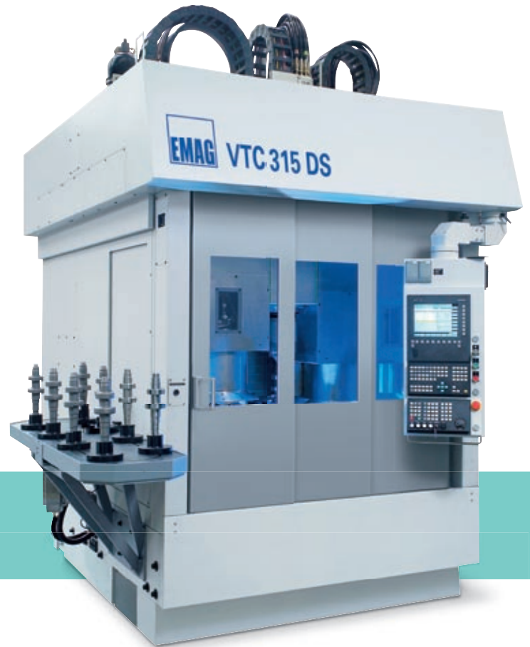
Automation integrated. A gripper in the turret ensures that the VTC 315 DS loads itself.
