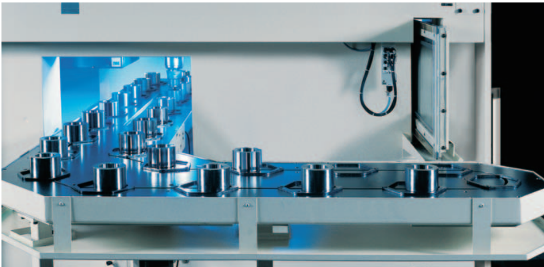
L-automation for stand-alone machines: The workpieces are conveyed to the pick-up station and the finish machined components removed
