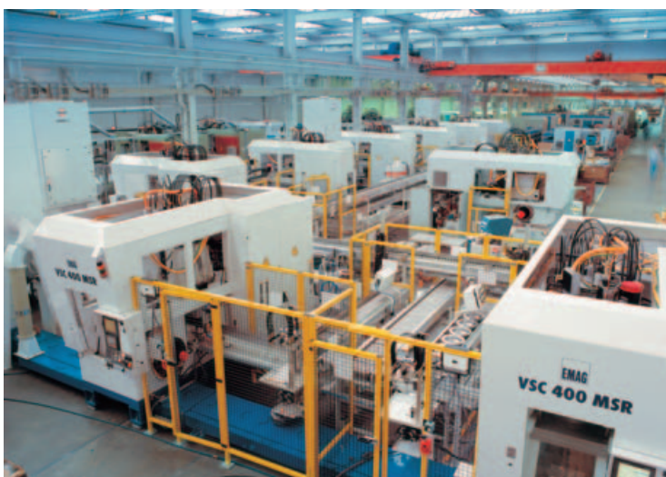
Multi-functional VSC production centers are frequently integrated into production lines, which then complete machine certain workpieces in the most sophisticated way. The picture shows 8 interlinked machines for the production of brake discs.
