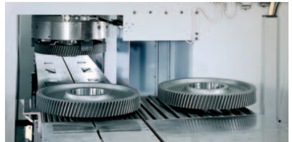
The workpieces are conveyed to the pick-up station and clamped by the spindle chuck
