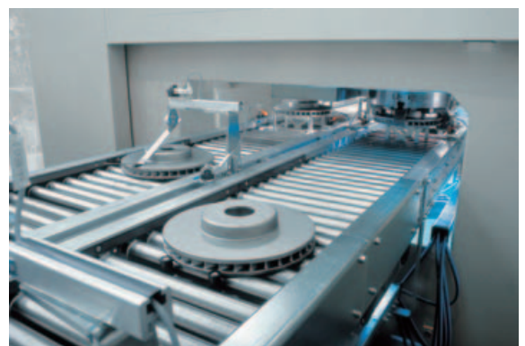
Twin-track load/unload for rapid workpiece changeover
