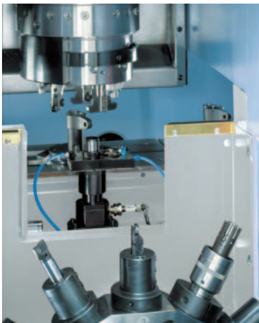
Measuring a bore with a plug gauge (Door between plug gauge and machining area open)
