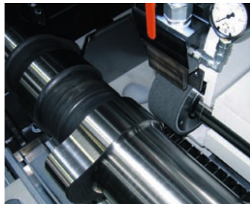
CBN-grinding of camshafts with concave radii
