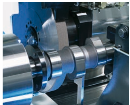
CBN-grinding of camshafts for railroad engines
