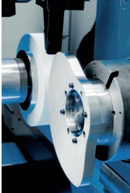
SK 204 machining area Grinding a radial cam
