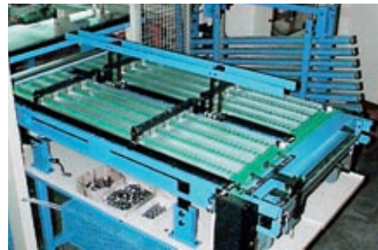
Long-time recirculating storage conveyor
