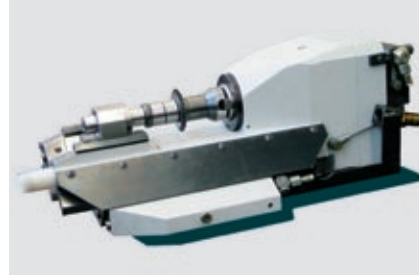
Shifting universal milling head for the hobbing of spur gears and the milling of single- and multi-start worms
