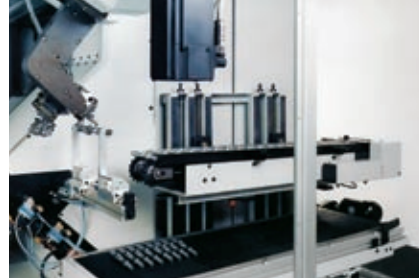
Integral gantry loader with flexible workpiece magazines, feeder chain and belt conveyor
