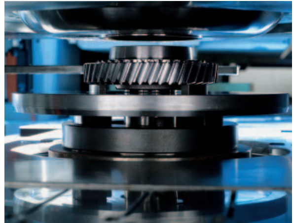
Optimised workholding technology ensures distortion is kept to a minimum.
